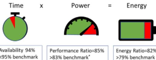
This PV System has a **lower PR** than an average of PR=83.5%\* while the average availability of 99% (over 7 years) is above the 95% benchmark. The following resources are available to help you optimize performance:
