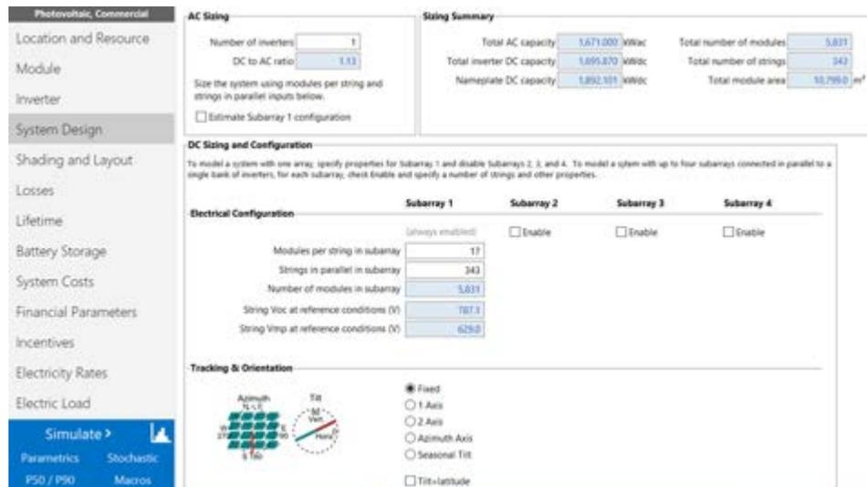
Figure 4. User interface for SAM used to predict modeled performance of each system.
